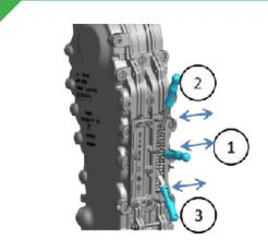
In case of watercircuit issues, the manifolds can be removed to clean each section individually
